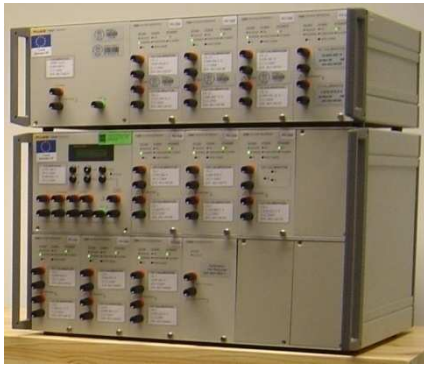
Figure 8. The group of ten solid-state references divided into the transfer module (above) and the maintenance module (below).
